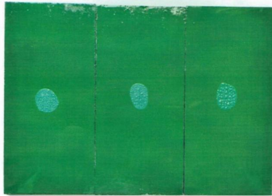
耐酸性 (10% H 2 SO 4 , 48h) 样品编号: W 202303291 Acid resistance (10% H 2 SO 4 , 48h) Specimen number: W202303291
